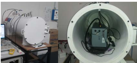
Aurora™ 4000 in a pressure chamber, testing the reliability when exposed to conditions expected at altitudes of up to 15,000 metres.
