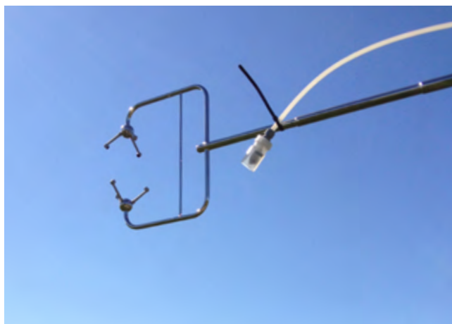
Figure 10. Sonic anemometer for REA measurements.
