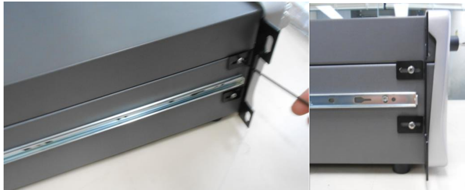
Figure 160 – Rack Mount Ears Fitted to Instrument
