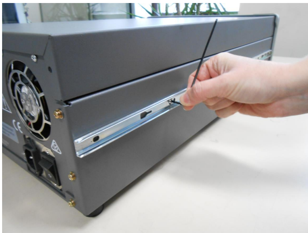
Figure 159 – Assemble Inner Slide on Chassis
