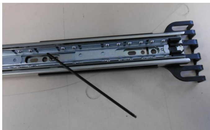
Figure 161 – Attach Rack Mount Adaptors to Outer Slides
