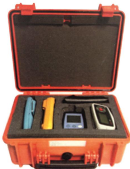
Figure 125 – Air Monitoring Test Equipment Kit (AMTEK) - Customisable
