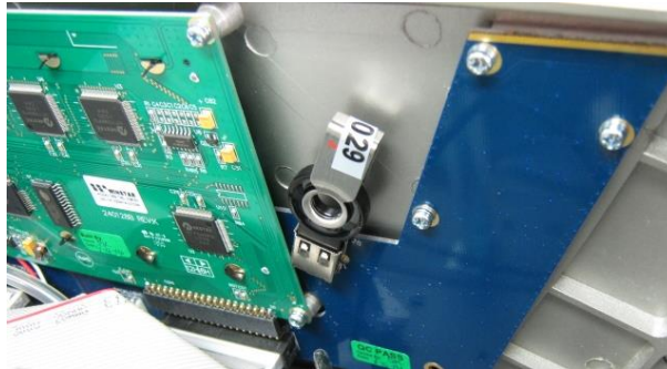
Figure 35 – Installation of USB Memory Stick
