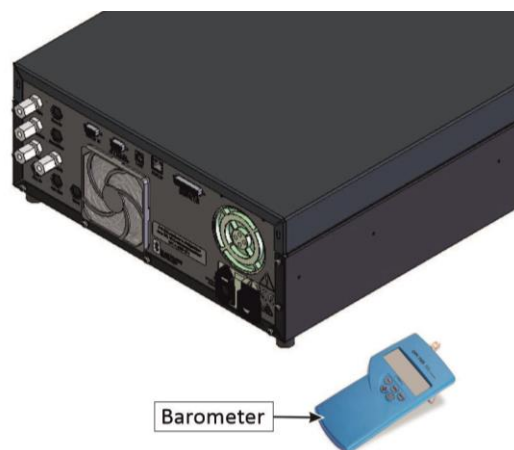
Figure 112 – Ambient Pressure Calibration Set-up
