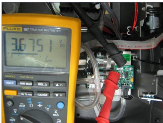
Figure 143 – Typical Test Point Reading of Manifold Pressure Sensor
