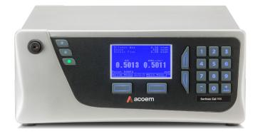
The Acoem Serinus° Cal 300 (formerly known as the Ecotech Serinus° Cal 300) includes a built-in ozone generator and internal zero-air source as well as a compact reference photometer, providing precise feedback control for accurate ozone generation and measuring in one unit.
