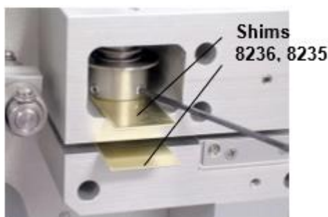
Figure 36 – Using Shims for Reassembly
