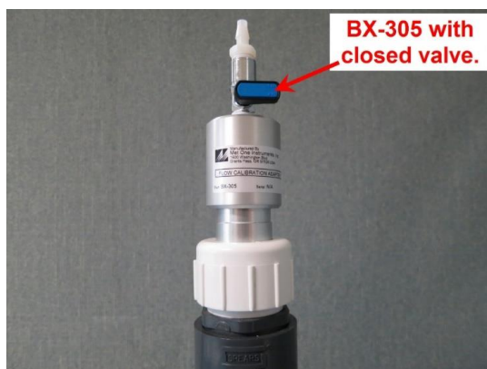
Figure 15 – BX-305 Leak Check Valve Installed on Inlet Tube
