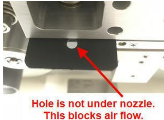
Figure 18 – Nozzle Seal Tool with Solid Side Under the Nozzle
