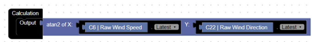
Logic Block Calculation Example
