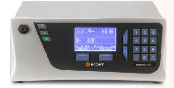
The Serinus® Cal 1000 performs gas dilution calibrations and is used in conjunction with regulatory traceable gases and a zero air generator.
