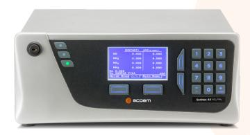
The Serinus<sup>®</sup> 44 analyser delivers precise and reliable performance at excellent value. It uses proven chemiluminescence technology and an external thermal catalytic converter to measure NO, NO<sub>2</sub>, NO<sub>x</sub> and NH<sub>3</sub> in ambient air.
