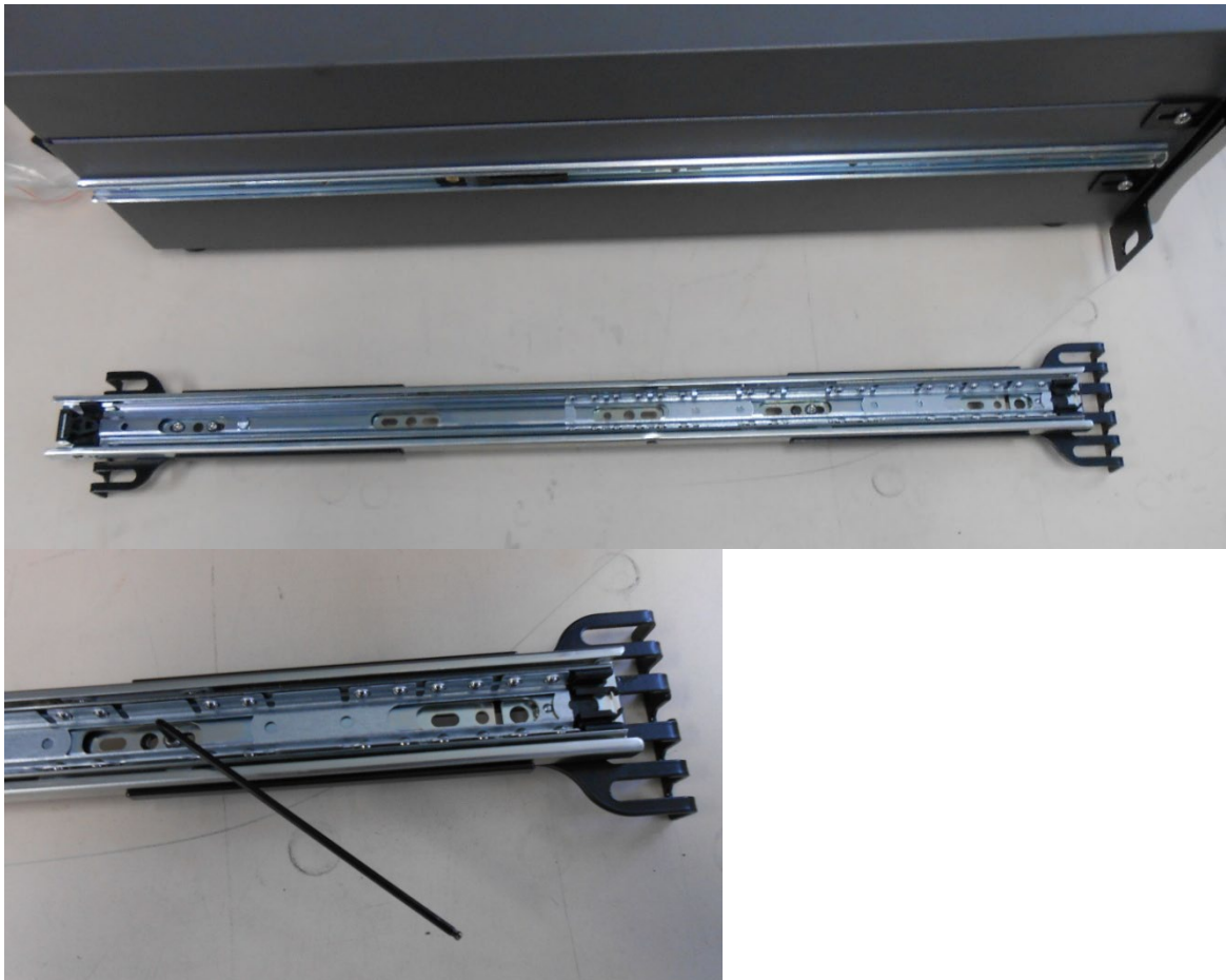
Figure 88 – Attach Rack Mount Adaptors to Outer Slides
