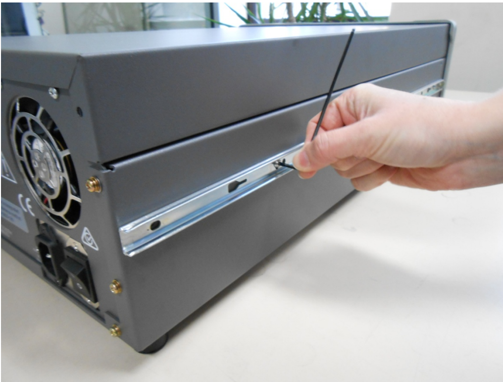
Figure 86 – Assemble Inner Slide on Chassis
