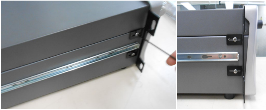
Figure 87 – Rack Mount Ears Fitted to Instrument
