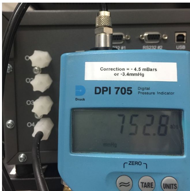
Figure 67 – Connecting the Barometer to O4 (Output 4)
