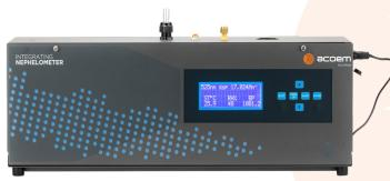
The Aurora<sup>™</sup> 2000 PM<sub>2.5</sub> Correlating Nephelometer is part of the new generation nephelometers, using a single wavelength and an LED light source to measure aerosol light scattering and derive particulate concentrations.
