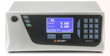
The Serinus<sup>®</sup> 50 sulfur dioxide  $(SO_2)$ analyser delivers precise and reliable performance at excellent value. It uses proven pulsed UV fluorescent radiation technology to measure  $SO_2$  in ambient air (LDL < 0.3 ppb, range 0 to 20 ppm).
