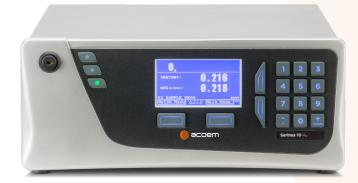
The Serinus® 10 Ozone (O<sub>3</sub>) analyser delivers precise and reliable performance at excellent value. It uses proven non-dispersive ultraviolet (UV) absorption technology to measure O<sub>3</sub> in ambient air (LDL < 0.5 ppb, range 0 to 20 ppm).
