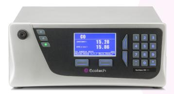
The Serinus<sup>®</sup> 30 carbon monoxide (CO) analyser delivers precise and reliable performance at excellent value. It uses proven NDIR gas filter correlation technology to measure CO in ambient air (LDL < 40 ppb, range 0 to 200 ppm).
