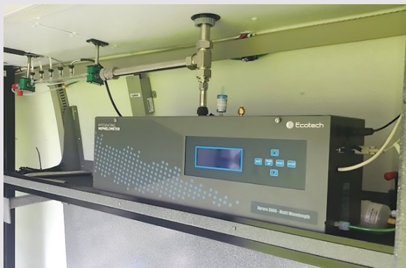
At the heart of the Ambilabs® Emergency Response Vehicle is the ECOTECH Aurora™ 3000 nephelometer.
