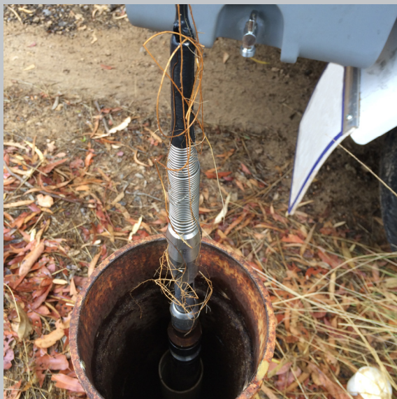
Pic above: The Portable Groundwater Profiling System (PGPS) designed by ECOTECH includes a winching system fitted with a sonde instrument probe to reach depths of 100 m and measures water quality at 1 cm intervals.
