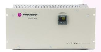
ECOTECH HTO-1000 Thermal Oxidiser is a thermal converter designed to be used with nitrogen gas analysers for the measurement of ammonia ( $NH_3$ ) or with sulphur dioxide gas analysers for the measurement of hydrogen sulphide ( $H_2S$ ) or total reduced sulphur (TRS).
