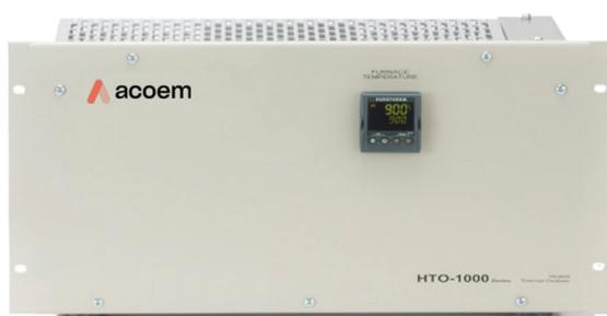
The Acoem HTO-1000 Thermal Oxidiser is a thermal converter designed to be used with oxides of nitrogen ( $\text{NO}_x$ ) gas analysers for the measurement of ammonia ( $\text{NH}_3$ ) or with sulphur dioxide ( $\text{SO}_2$ ) gas analysers for the measurement of hydrogen sulphide ( $\text{H}_2\text{S}$ ) or total reduced sulphur (TRS).
