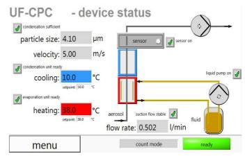
Figure 3: Touch screen user interface showing device status
