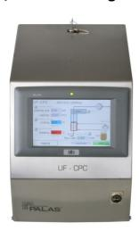
The Palas® condensation particle counter UF-CPC is available in three models, each of them being optimized for a different concentration range. Model 50 is optimized for low concentrations (e.g. after a filter or in an hospital operating room), whereas model 100 is appropriate for medium concentrations (e.g. ambient monitoring). Model 200 offers single particle counting up to 1,000,000 particles/cm³ (e.g. for printer emission studies).
