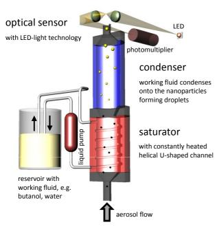
Figure 2: Working principle of the universal fluid condensation particle counter (UF-CPC)
