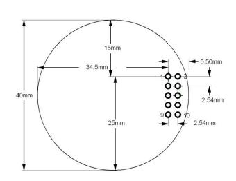
Note that the drawing shows details of the PCB inside the sensor casing. The outside dimension of the sensor casing is 43mm.
