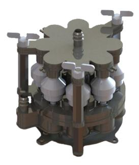
Miniaturized eight-channel filter sampler for timeresolved aerosol chemistry measurements
