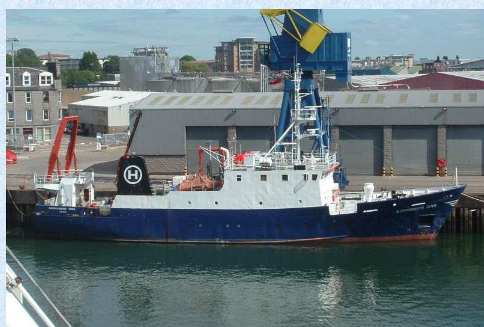
Fig. 2. The Commandor Iona vessel where all the instruments were hosted. Sampling containers were installed in the front of the ship to avoid contamination from the ship's stack emissions.
