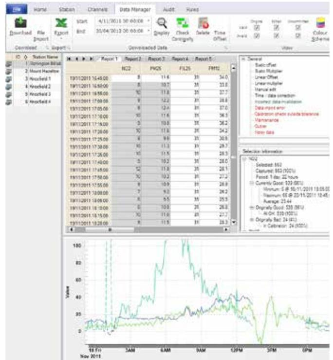
Data is presented onscreen in a fully configurable table and in a zoomable dynamic graph. Data selected in the graph is also selected in the table and vice versa. This allows for blocks of data to be quickly examined and individual measurement peaks to be scrutinised.
