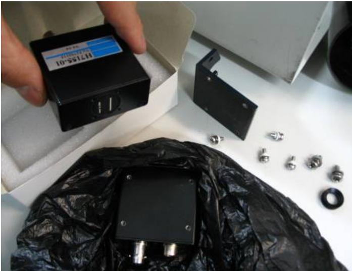
**Figure 50 – New PMT inserted**
