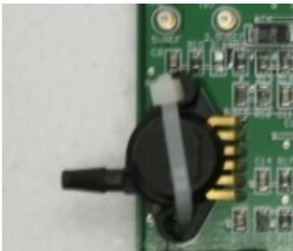
**Figure 13 – Pressure sensor**
