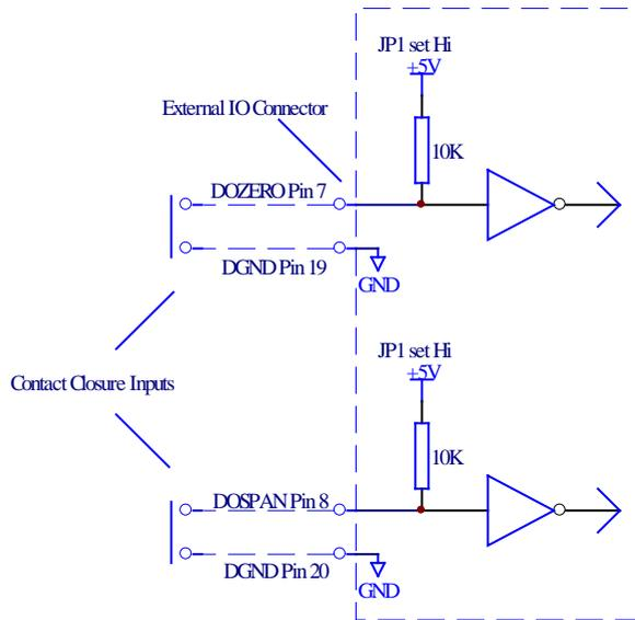
**Figure 27 – External span & zero control**
