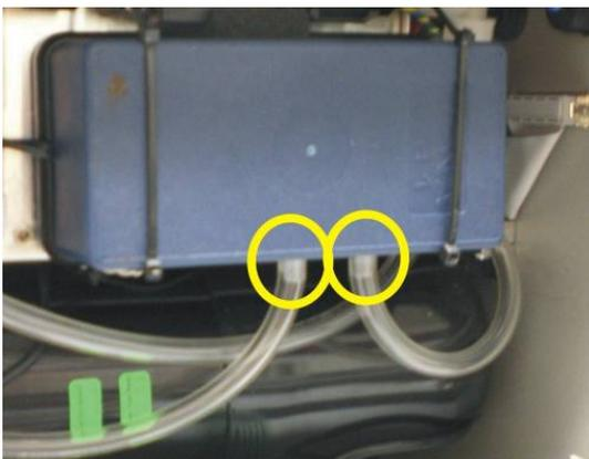
**Figure 56 – Pump ports**
