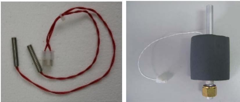
**Figure 14 – Cell & inlet heaters**
