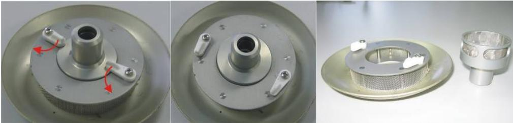
**Figure 42 – Insect trap removal**
