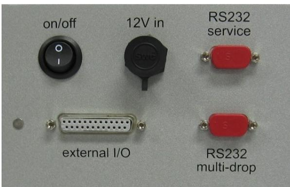
**Figure 17 – Electrical connections to Aurora 1000**
