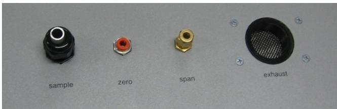
Figure 18 – Pneumatic connections to Aurora 1000
