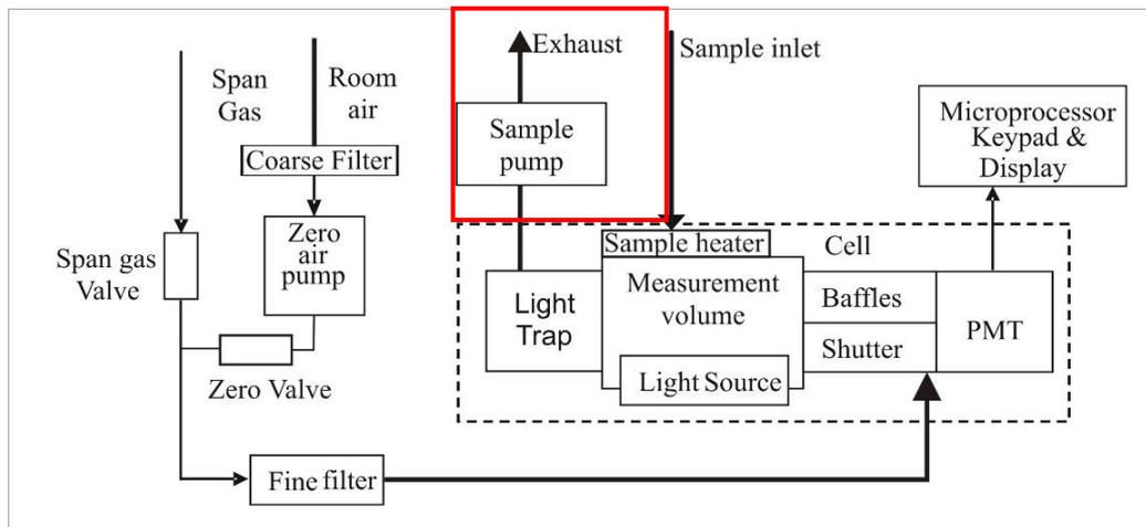
**Figure 51 – Aurora 1000 block diagram (red box shows changed pneumatics)**
