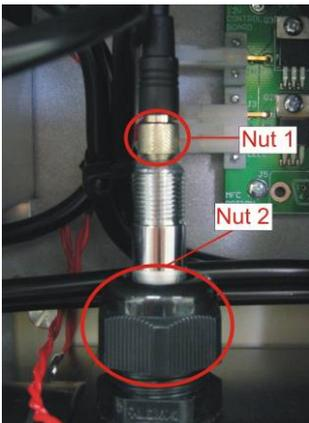
**Figure 26 – Temperature/humidity sensor**
