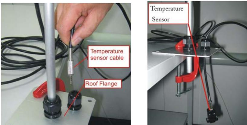
Figure 60 – Installing the ambient air temperature sensor stage 2
