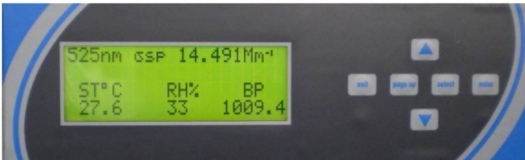
Figure 23 – Display panel & keypad
