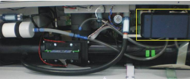
**Figure 54 – Pump bracket**
