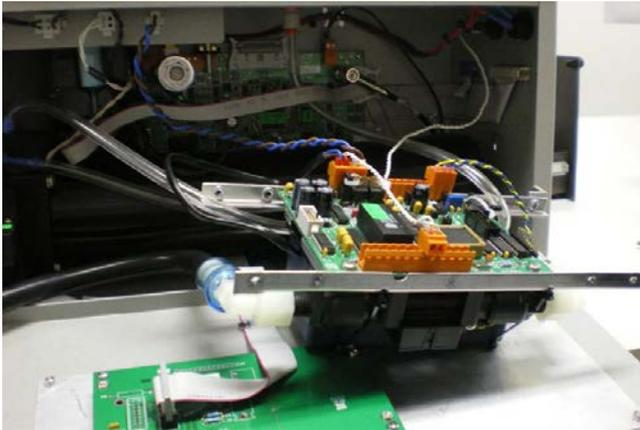
**Figure 55 – Pump bracket removed from nephelometer**
