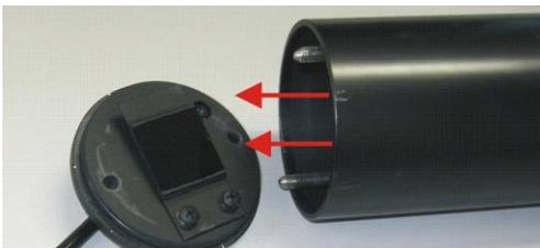
**Figure 48 – Removing light trap**
