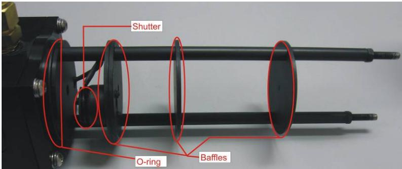
**Figure 46 – Optical chamber right cylinder components**
