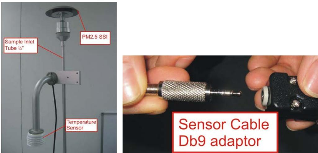
Figure 59 – Installing the ambient air temperature sensor stage 1
