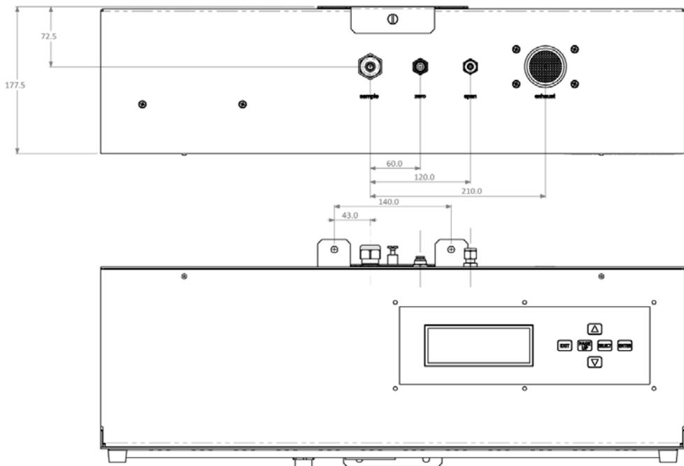
**Figure 22 – Locations of pneumatic ports**
