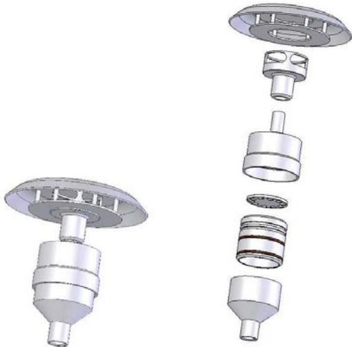
**Figure 57 – PM<sub>2.5</sub> inlet collapsed and expanded**
