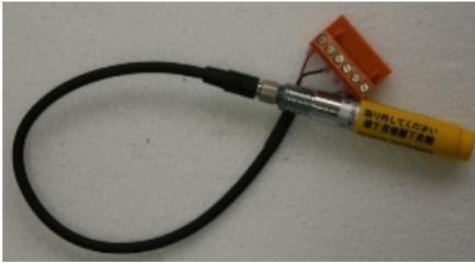
**Figure 12 – Temperature/RH sensor**
