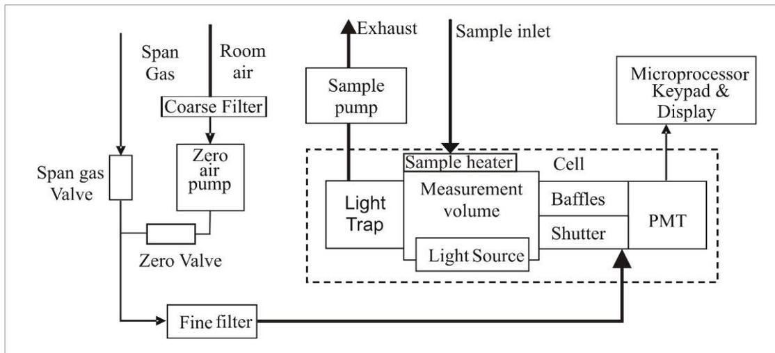
**Figure 2 – Block diagram**
