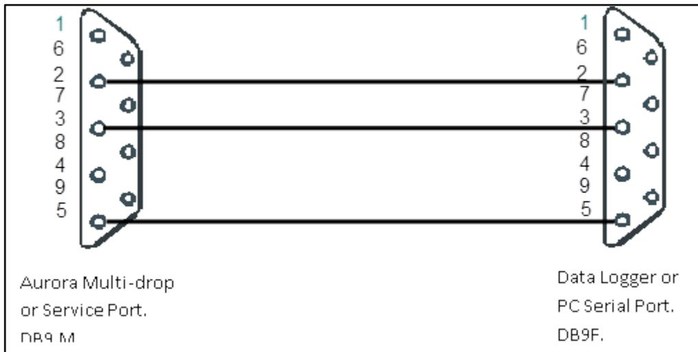
**Figure 20 – Aurora service & multi-drop serial port cable**
