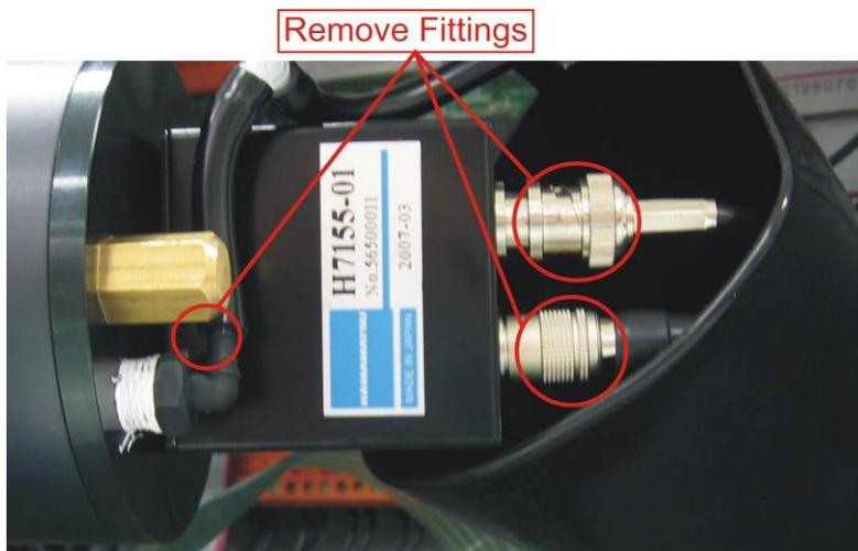
**Figure 45 – Removal of cell fittings**
