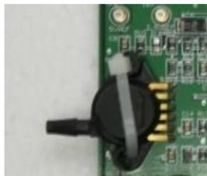
Figure 15 Pressure sensor
