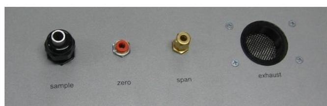
**Figure 20 Pneumatic connections to the Aurora 4000**
