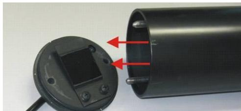
**Figure 49 Removing Light Trap**
