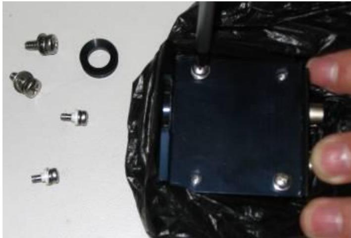
**Figure 45 Removing the PMT**
