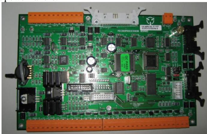
**Figure 17 Microprocessor board**
