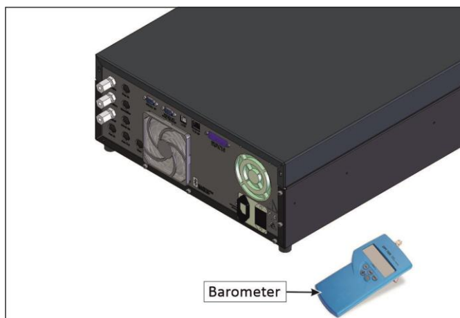
Figure 104 – Ambient Pressure Calibration Set-up
