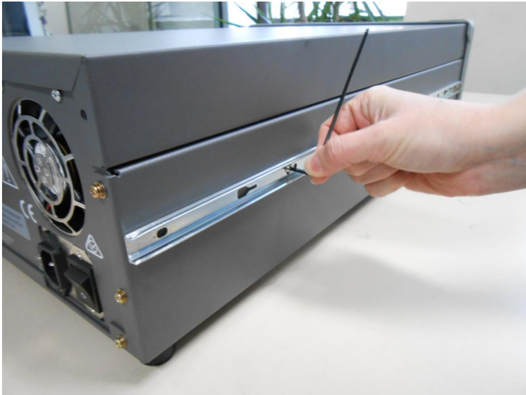
Figure 151 – Assemble Inner Slide on Chassis
