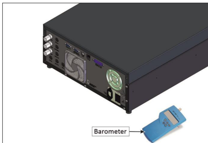
Figure 103 – Full Pressure Calibration Set-up (Ambient)
