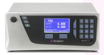
The Serinus<sup>®</sup>57 Total Reduced Sulfur analyser delivers precise and reliable performance at excellent value. It uses proven UV luorescent radiation technology and a thermal converter to measure TRS in ambient air (LDL < 0.3 ppb, Range 0 - 2 ppm).
