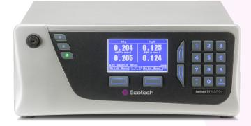
The Serinus® 51 analyser delivers precise and reliable performance at excellent value. It combines pulsed fluorescence detection with an internal catalytic converter to sequentially measure H<sub>2</sub>S and SO<sub>2</sub>in the range of 0 - 2 / 0 - 20 ppm respectively with a detection limit of 0.3 ppb.
